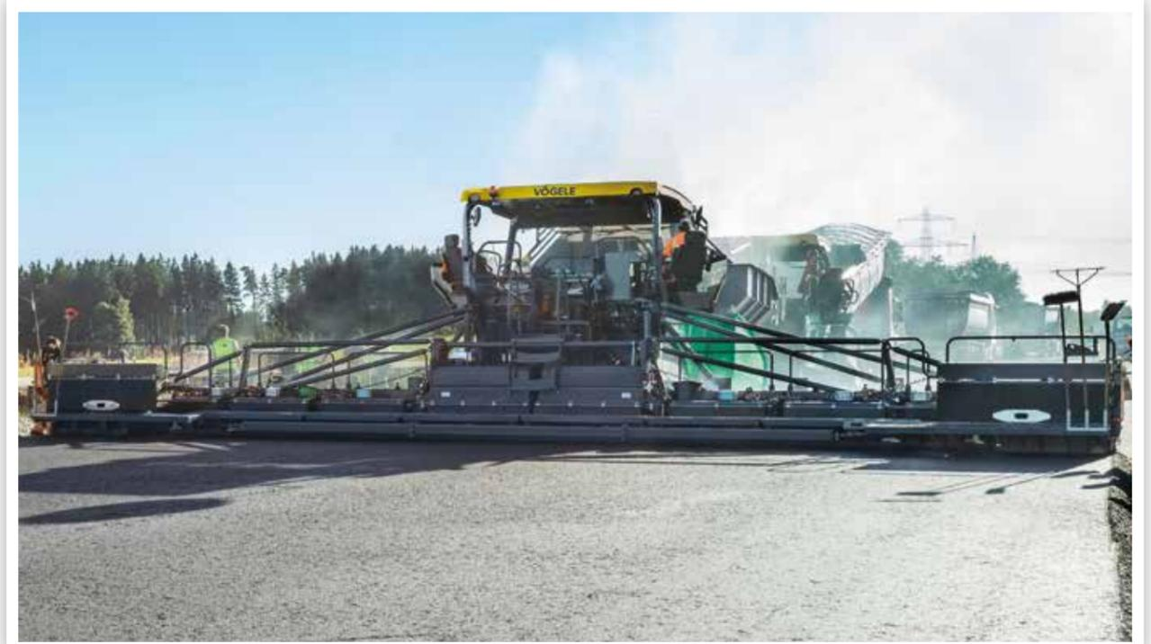
**With a pave width of up to 18m**, a maximum laydown rate of 1,800t/h and an engine output of 354kW, the SUPER 3000-3 is the new flagship in VÖGELE's paver line-up. As a representative of the Premium Line, this large paver incorporates all the features of the "Dash 3" generation.
