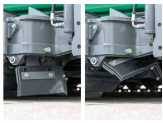
The sturdy deflectors in front of the crawler tracks reliably clear any spilled mix out of the way. They can be hydraulically raised or lowered automatically at the press of a button or using the AutoSet Plus.
