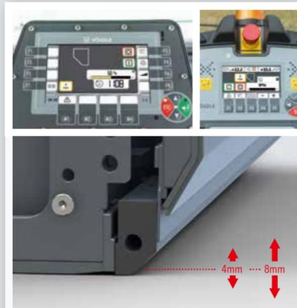
**Hydraulic Tamper-stroke adjustment
