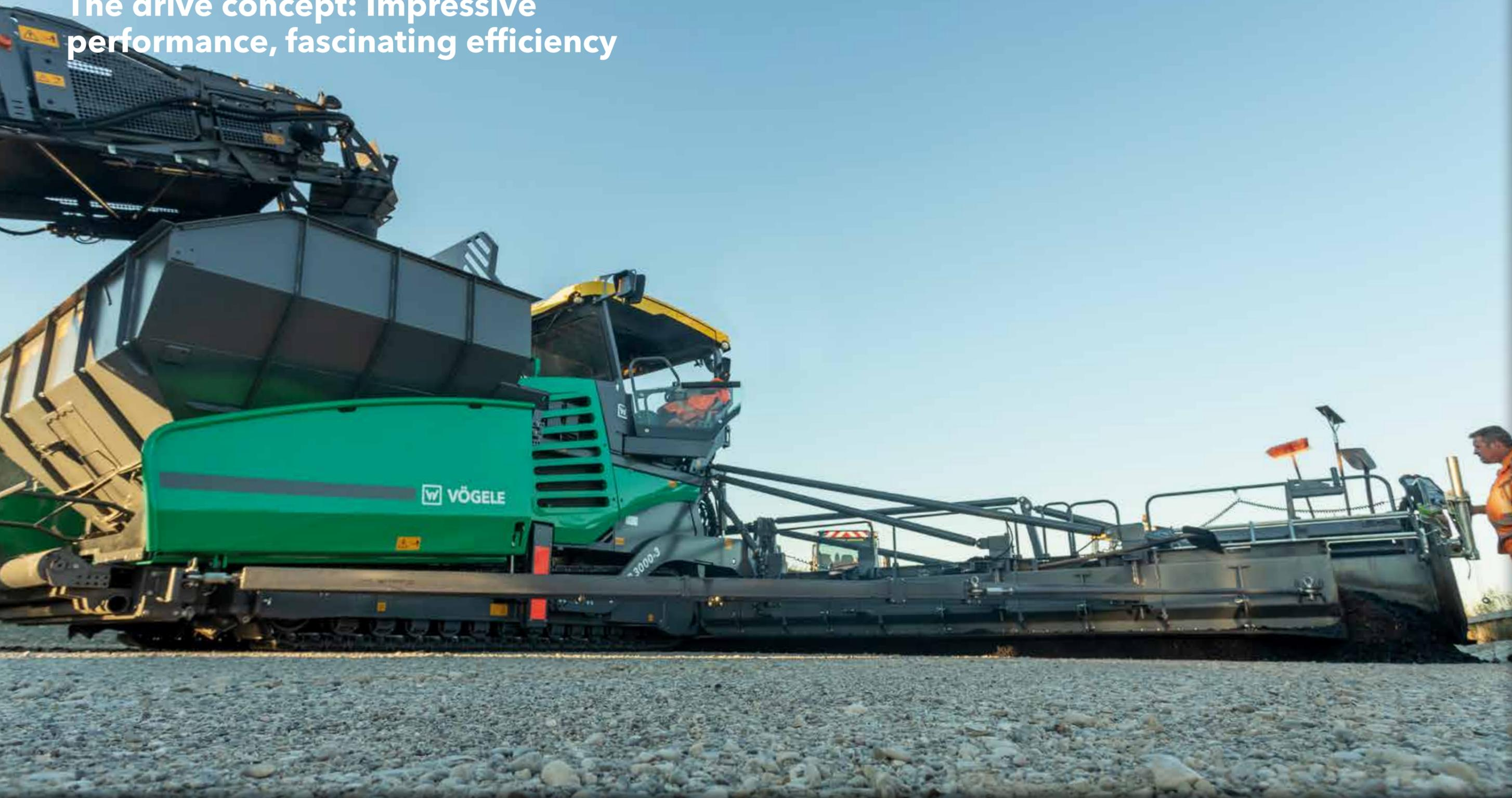
**The powerful 6-cylinder diesel engine** rated at 354kW is the driving force behind the Highway Class paver.
