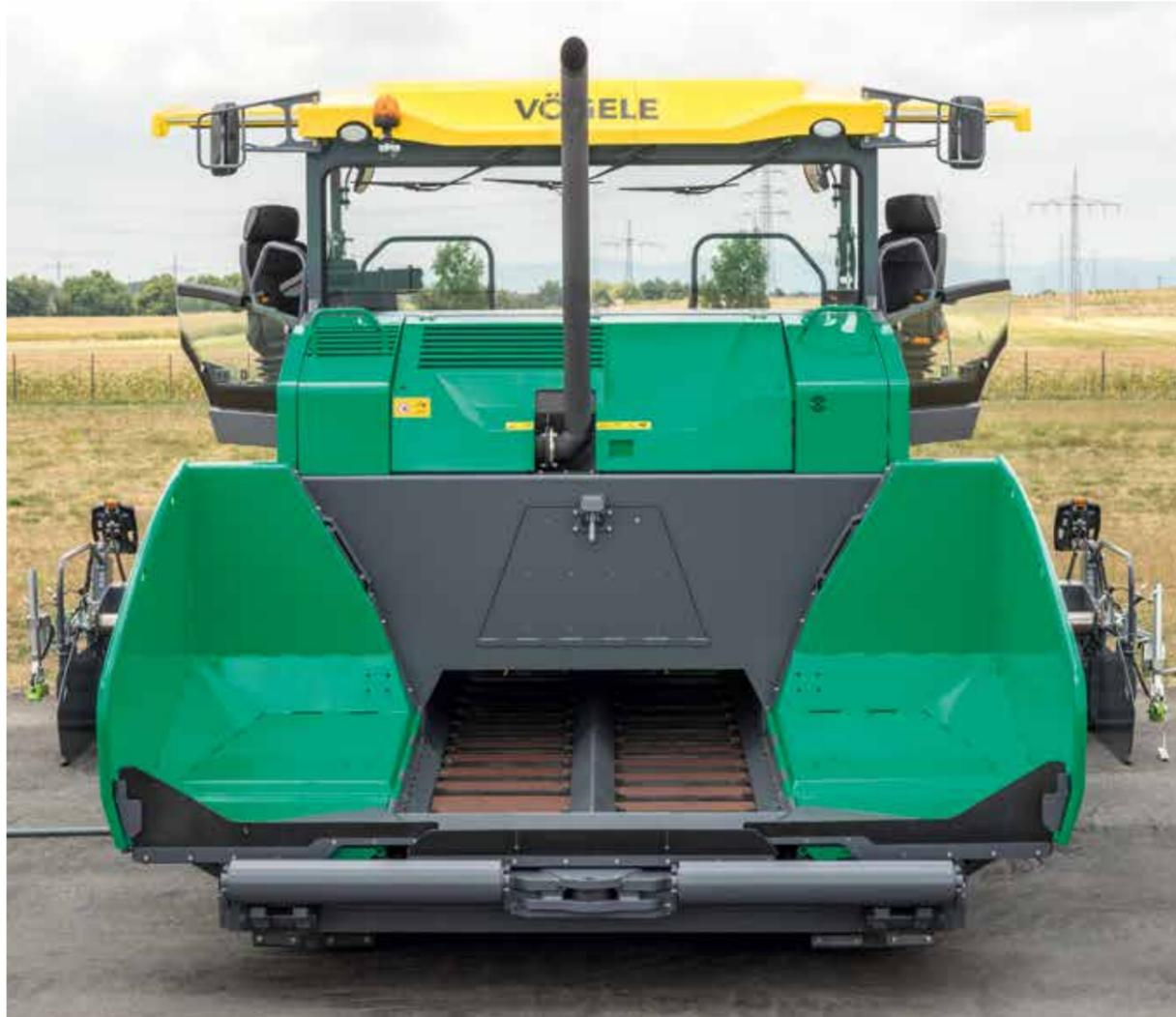
» **The huge material hopper** has a capacity of 18.5t, allowing feed lorries to be emptied in a very short space of time.
